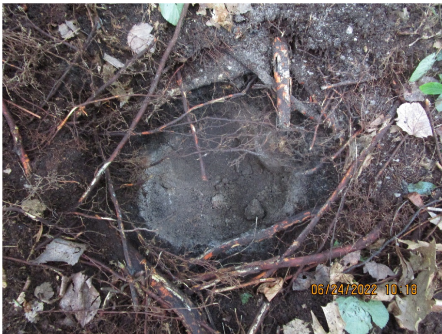
Photo 3 – 18" Deep Test Hole with Ashy-Grey colored silt / gravel (dry)
