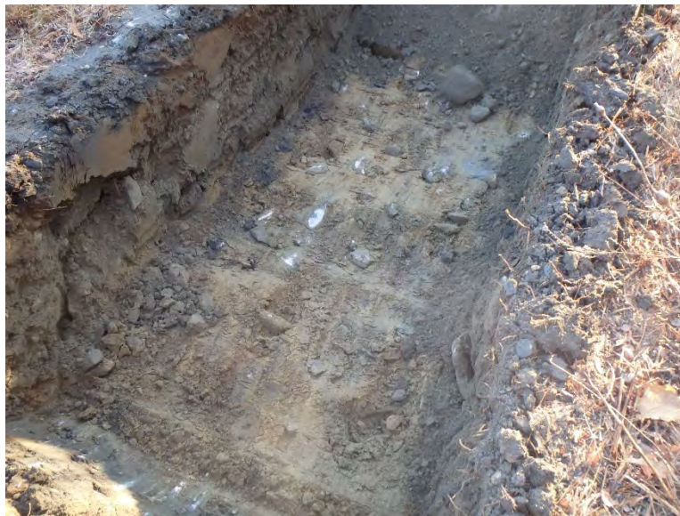
Photograph 3. Exposed fills at 1meter (3.3 feet) below surface.
