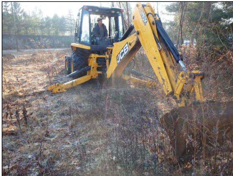
Photograph 2. JCB 3CX backhoe with flat edge bucket.
